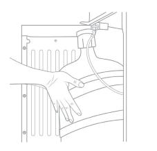
8. Push the head down until the tube hits the bottom of bottle.
