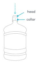
7. If you are using a 3 gallon bottle rather than a 5 gallon bottle you can adjust probe by pressing the two tabs at the head of the probe and sliding the collar down to the neck of the bottle.
